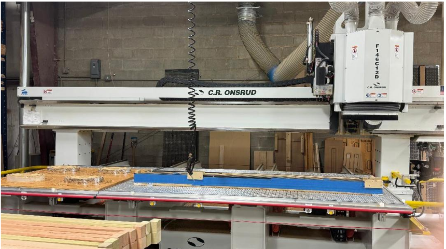
This Onsrud machine is cutting tapered 8 sided pencil post bed posts; it's a "set it up, put your wood on the table in precise locations, turn it on, and walk away. A time saver when doing sizeable complex runs.
