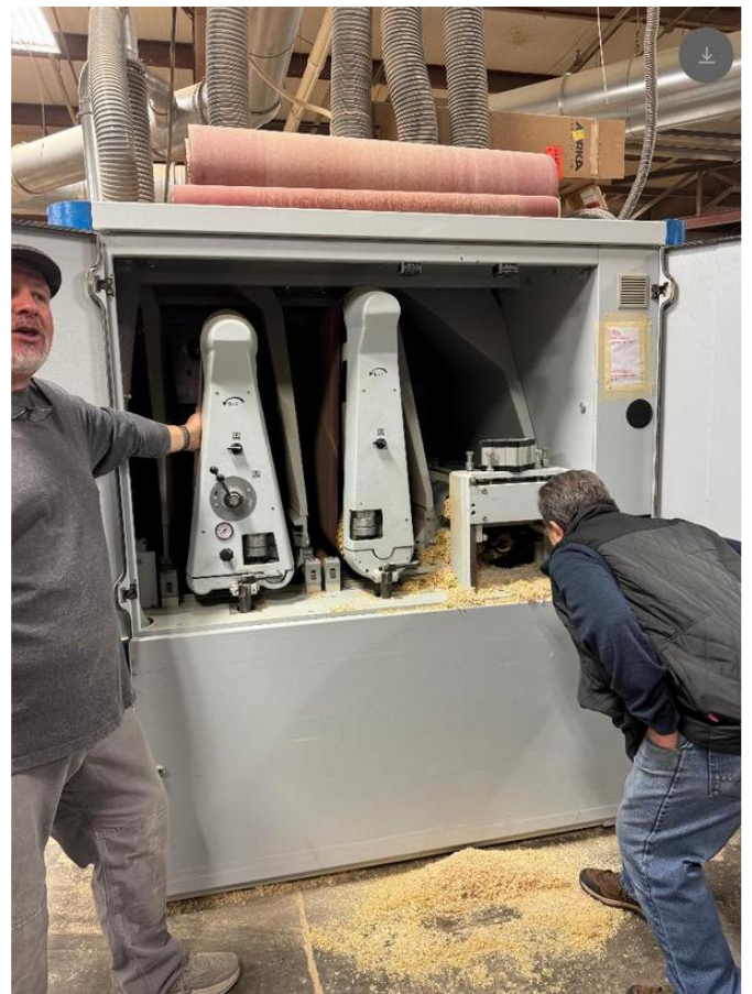
Wide board planer and double grit sander all in one pass; another big time saver.
